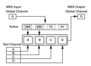
The global channel acts just like playing on the keyboard. The individual slot channels give multi timbrality. MIDI output is always sent on the global channel.
