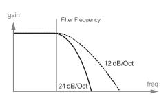
has a steeper slope than a 12 dB/octave.
