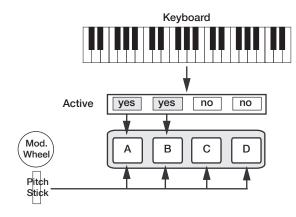
All active Slots respond to keyboard input. Modulation Wheel, Pitch Stick and Control Pedal always reach all slots.
