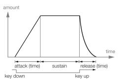
turned fully clockwise, the decay will be infinite, acting as a sustain level. *Range: 3.0 ms to 45 s, Sustain.*
